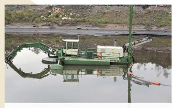
Dredging Systems Pty Ltd was engaged to remove the sludge so that the coal fines could be recovered. A small dredge was used with a rotating cutting head on the inlet pipe. This enables the sludge to slurry in the base of the pond and enables the collection of solids to be accelerated.
